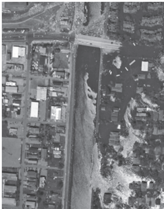
Fig. 10. Vertical air photograph of the 17th Street Canal, with its failed eastern levee (on the right) releasing the major flood flow into the city; at the top of the picture floating debris is trapped behind the bridge over the inflow from Lake Pontchartrain, while the urban area west of the canal remains dry. (Photo by NOAA)
